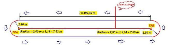
Total length = Radius A 7,53 m + Radius B 7,85 m + 492,30 x 2 = 1.000 Meter
